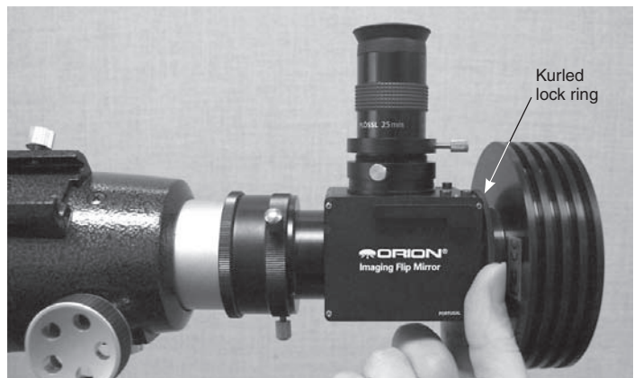
Figure 4. Use the knurled lock ring to secure the camera orientation.
