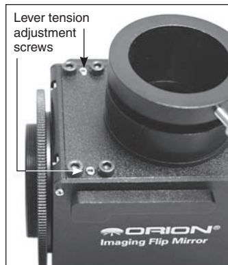
Figure 6. (above) The two silver socket head screws located above the lever adjust the lever tension.
