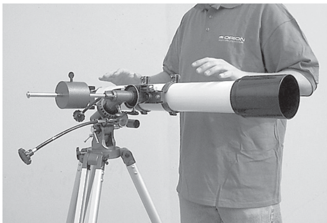
Figure 3e. Telescope is now balanced on the Dec. axis, i.e., it remains horizontal when hands are released.
