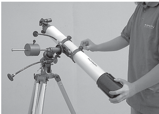
Figure 3d. Balancing the telescope with respect to the Dec. axis. As shown here, the telescope is out of balance (tilting).
