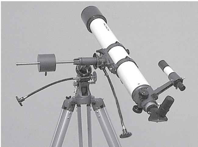
Figure 5a. Telescope pointing south. Note that in all these illustrations, the mount and tripod remain stationary; only the R.A. and Dec. axes are moved.
