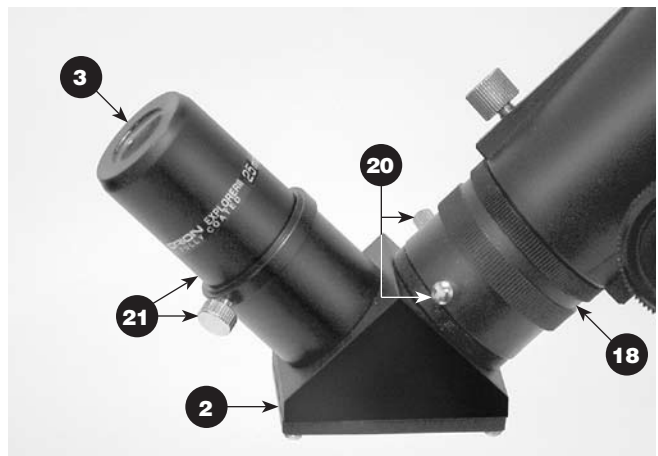
Figure 2b. Observer 70 focuser detail
