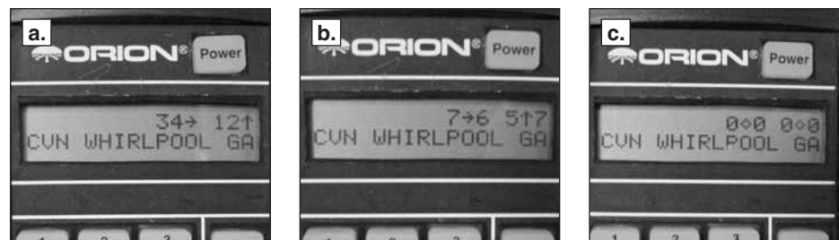
Figure 11. This sequence of pictures illustrate how the controller's guide arrows will look as you are finding an object. (a.) When you are far away from the object, there will be a number (from 10 to 179) to the left of the guide arrows. (b.) When you are close to the object, each guide arrow will display a number on its immediate left (from 0 to 9) and immediate right (from 0 to 9); the number on the left is whole number increments, while the number on the right is in increments of tenths. This helps in making small movements to the telescope to pinpoint the object's location. (c.) When the guide arrows display "0.0 0.0", the object will be within the field of view of the telescope (with a 25mm or longer focal length eyepiece).
