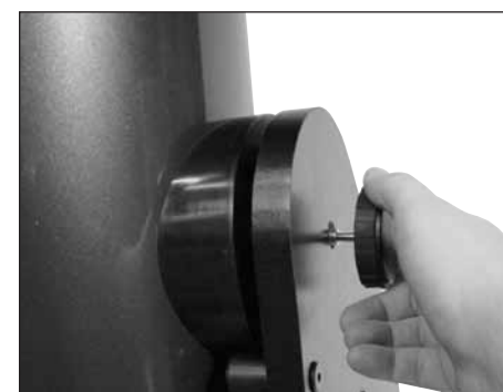
Figure 7. The retaining knob goes through the shaft of the altitude encoder assembly before threading into the side bearing on the telescope tube.
