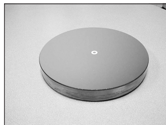
Figure 6: The primary mirror's center is now marked, and it is ready to be reinstalled.
