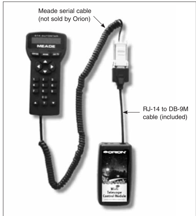
Figure 1. Connecting the Wi-Fi Module to a non-Orion GoTo controller requires a serial cable for that brand/model.
