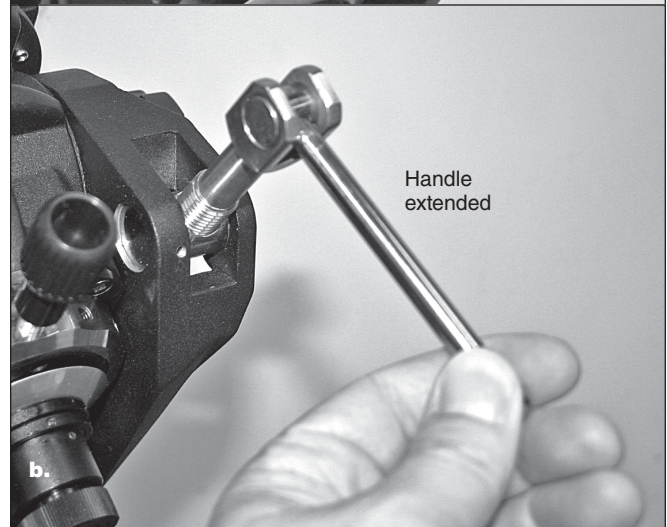
Figure 13. The altitude jackscrew with handle a) retracted, and b) extended for turning.
