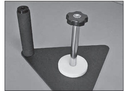
Figure 2. Loading counterweights onto, and removing counterweights from, the Counterweight Carrier is best done with the Carrier in this orientation.
