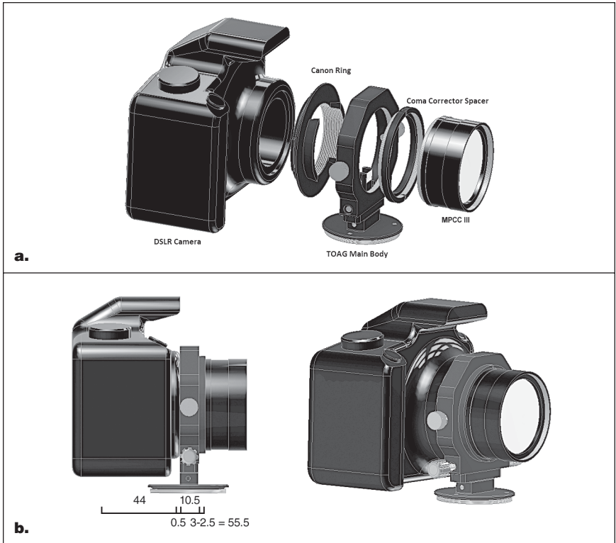
Figure 6. a) DSLR Camera with TOAG and MPCC spacer, b) Coma-corrector at the required distance to the camera sensor.
