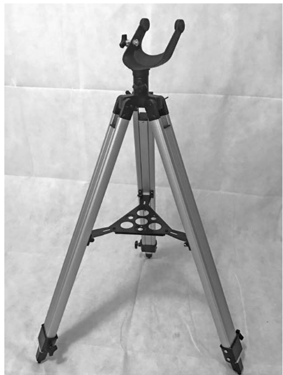
Figure 6. The assembled altazimuth mount and tripod.
