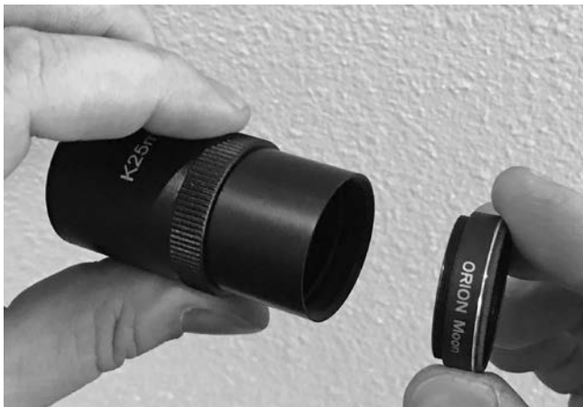
Figure 13. The Kellner eyepieces have barrels threaded to accept optional Orion 1.25" filters. A Moon filter is useful for cutting glare and revealing more detail on the lunar surface.
