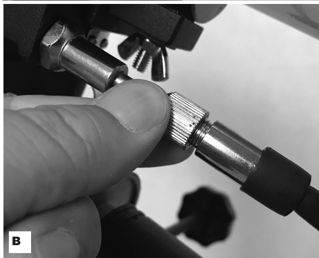
Figure 8. A) Slide the slow-motion cable onto the gear shaft as shown, B) then thread the knurled nut into the threaded end of the cable until tight.
