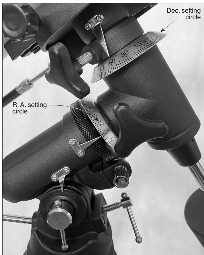
Figure 14. The R.A. and Dec. setting circles allow you to locate an object by its R.A. and Dec. coordinates.
