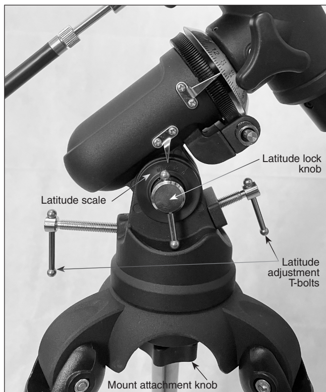
Figure 13. Loosen the latitude lock knob, then use the two latitude adjustment T-bolts to set the latitude scale pointer to your location's latitude.
