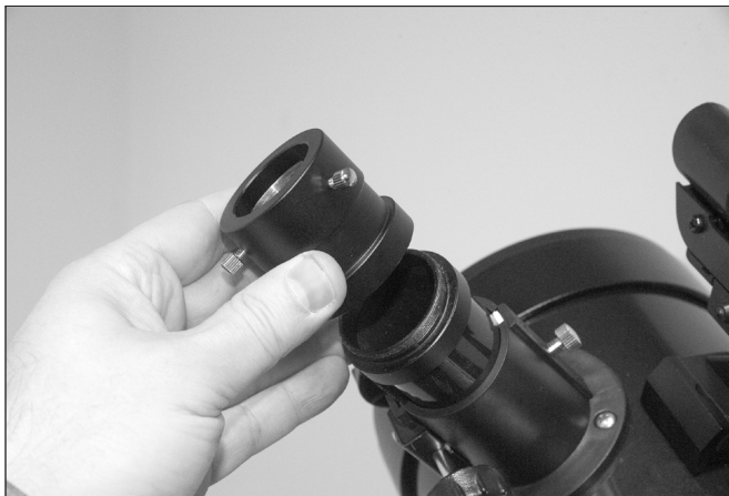
Figure 7. The Visual Back (eyepiece adapter) threads onto the focuser drawtube.
