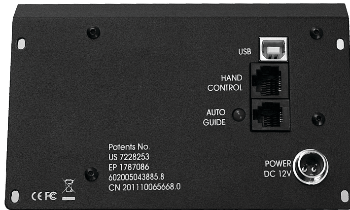
Figure 1. A USB Type B port has been added directly above the Hand Control port on the electronics panel.
