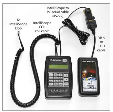
the local Wi-Fi connection between the Wi-Fi module and your iPhone, iPad, or iPod Touch, and you have completed the two-star alignment using the IntelliScope COL, you will no longer use the COL for object location. But it must remain powered on!
